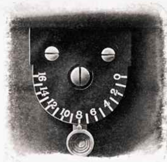
PLATE No. 6. PRESSURE INDICATOR.
