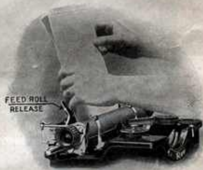
Inserting Several Sheets with Feed-Rolls Released
