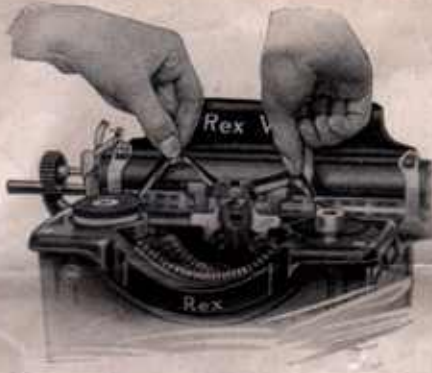
Inserting Ribbon—Drawing It Into Upper Guide Loops on Vibrators
