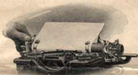
Pressing Carriage Release to Give Free Movement to Right or Left
