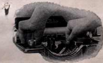
Inserting Ribbon—Sliding It Edge Down Into Lower Guide Loops
