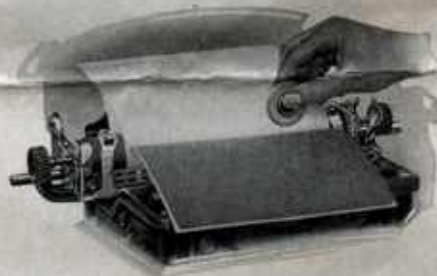
Erasing Carbons—A Card Placed Behind the Sheet Erased Prevents Blurring
