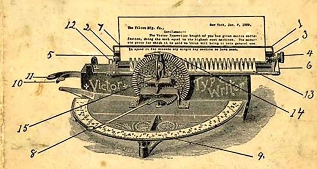
Bring the bail or wire rod (1) forward as near the type-wheel as possible, place the paper squarely into the carriage (2) from the back of the machine, moving the paper forward and upward under the rubber roll (3), turn from you the milled head (4) at the right of the carriage, and the paper will be raised in front of the bail-rod; push the bail-rod back against the paper, to keep it (the paper) in an upright position against the printing surface (5).
