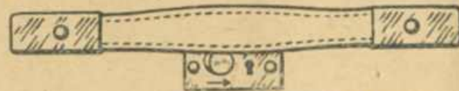
Turn key to the right, and knob pressed in direction of the arrow.
